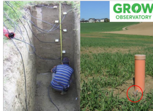
Figure: Two different examples of in situ sensors (left hand side – professional sensor in several depths; right hand side – low cost sensor in red circle next to professional sensor).
