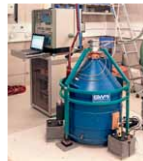
Superconducting gravimeter (in blue) at the Conrad Observatory
