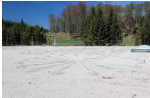
Starlike geometric configuration at the infrasound test field located south-west of the SGO.
