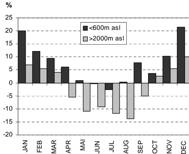
Mean annual course of the breaks in Austrian sunshine series due a change from the traditional Campbell-Stokes recorders to the Haenni-Solar sensors (new minus old in %, sample 1986-1999, dark: mean of 4 low-level sites, light: mean of 3 high-level sites)
