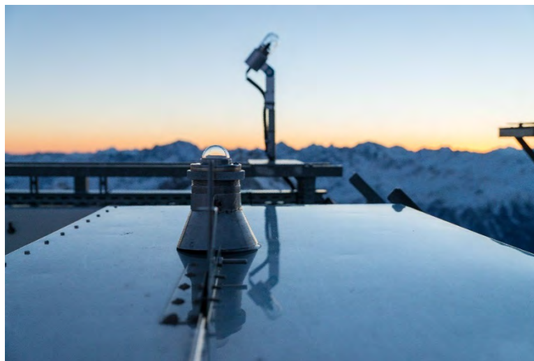
Figure 9 The Bentham spectrophotometer at sunset at the High Alpine Observatory Hoher Sonnblick (3106 m).
