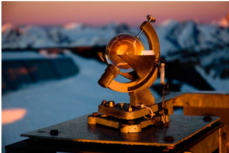
Figure 5 The Campbell-Stokes sunshine recorder at station Sonnblick.
