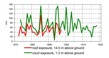
Figure 4: Example for inhomogeneities: Exposure of instruments
